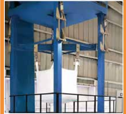
Load Testing machine
